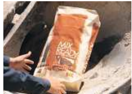
Disintegrating bags with powdered pigments are increasingly popular among ready-mix producers. The pre-measured bags can be thrown into mixers without opening or pouring and are a clean and convenient way to color ready-mix concrete.
