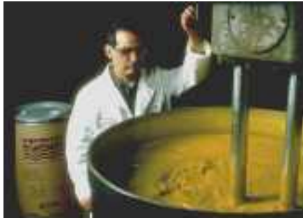
Liquid colors, also called slurries, are manufactured by mixing powdered pigment and dispersing agents in water using high-shear blenders.
